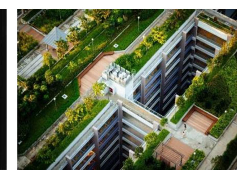
Fig.4 Vertical Greenery / Rooftop greenery - planting of greenery on vertical walls and rooftops to increase rainwater retention, resilience to heat etc.
