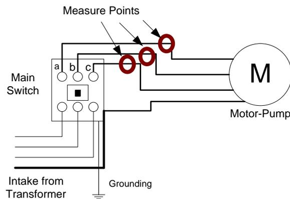
**Figure 5: Electrical Current Measurement**
