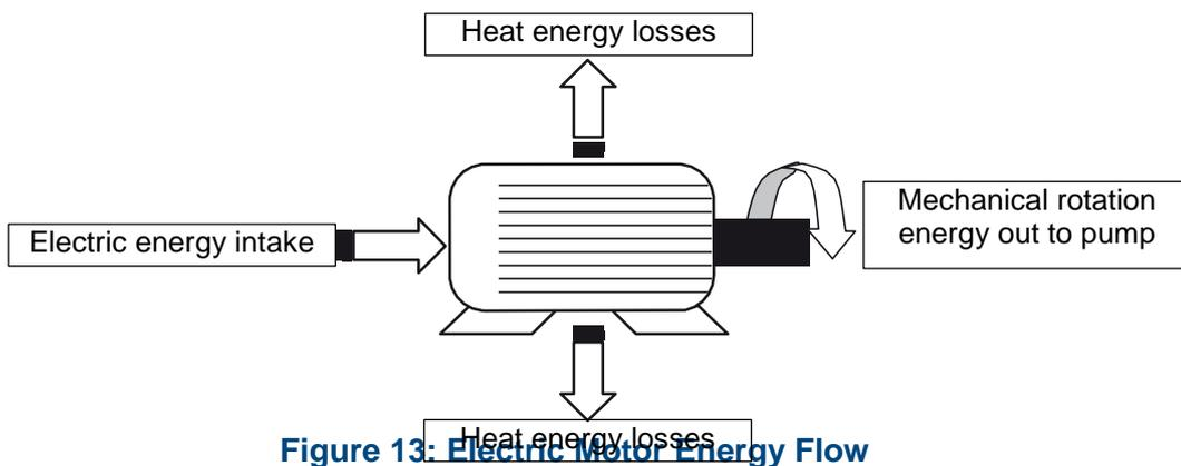
Figure 13: Electric Motor Energy Flow
