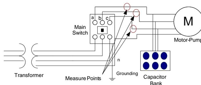
Figure 6: Measuring the Real Power before the Capacitors Bank
