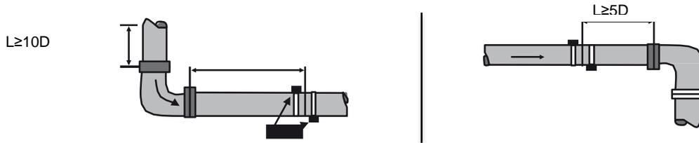
**Figure 8: Position of the Flow Meter**
