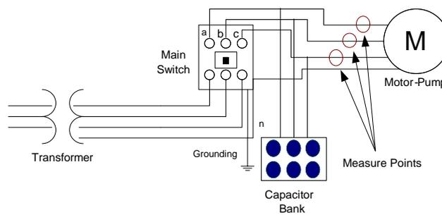
**Figure 7: Measuring the Real Power after the Capacitors Bank**
