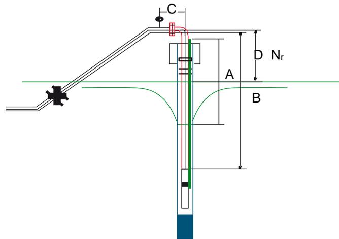
**Figure 12: Submersible Pump Level Measurement**
