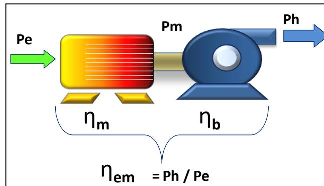
**Figure 18: Efficiencies that Comprise the Electromechanical Efficiency**
