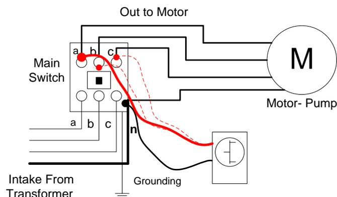
**Figure 4: Measurement of Voltage in Pumping Equipment**
