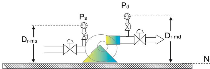
**Figure 11: Measurement of Pressure When Gauges in Suction and Discharge Are Available**
