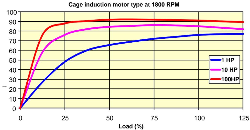
**Figure 14: Typical Efficiency vs. Load Curves for an 1800-RPM Cage Induction Motor**
