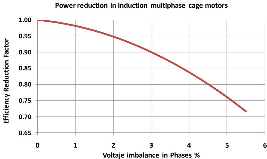
**Figure 16: Reduction in the Capacity of an Electric Motor Based on the Voltage Imbalance**
