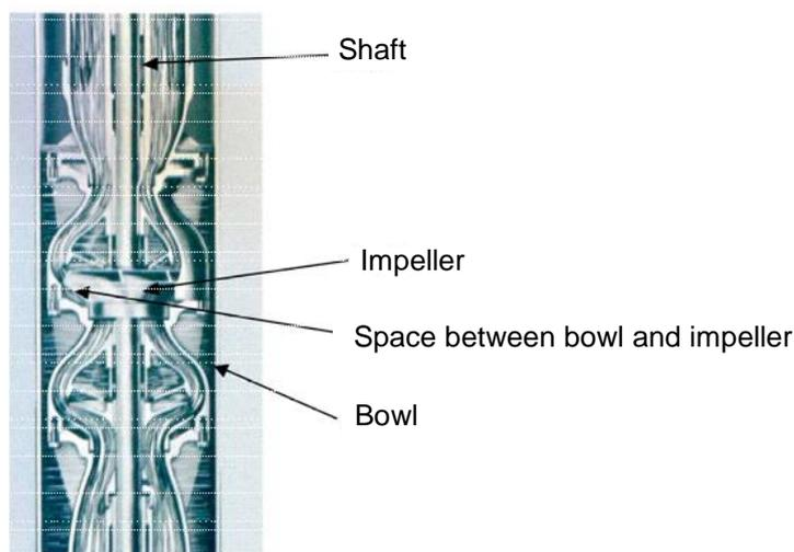
**Figure 20: Turbine Pump with Open Impeller Diagram**
