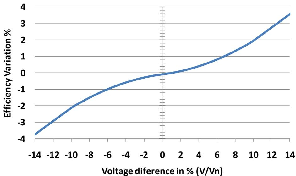
**Figure 15: Efficiency Variation Based on the Difference with Respect to the Original Voltage in an Electric Motor**
