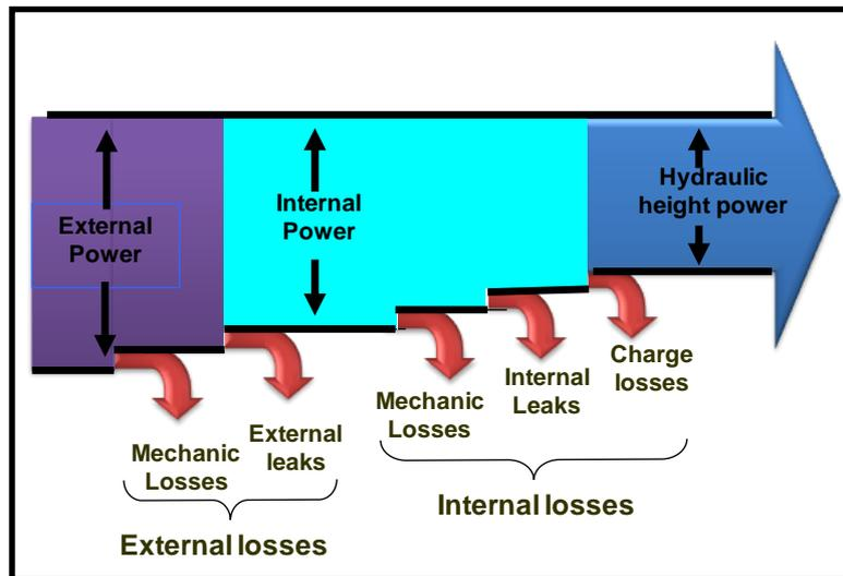
**Figure 17: Losses in Centrifugal Pumps**
