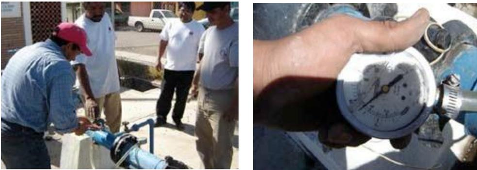
**Figure 9: Pressure Measurements with a Bourdon Type Gauge**
