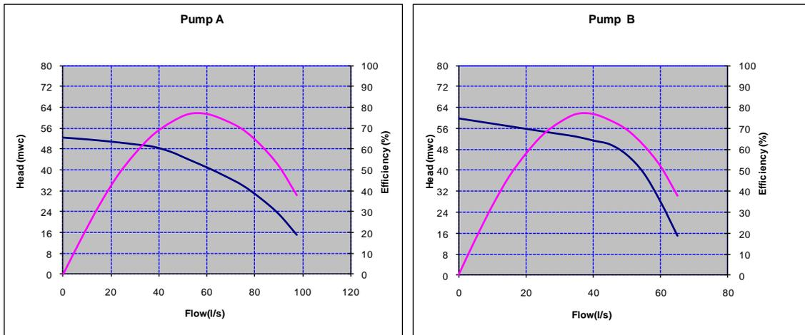
**Figure 19: Typical Curves of Two Pumps with Different H-Q Operation**
