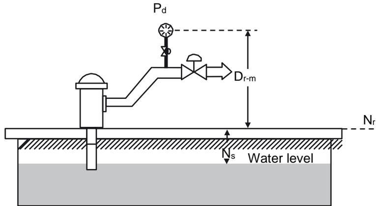
**Figure 10: Measurement for Pressure Gauge in the Discharge**
