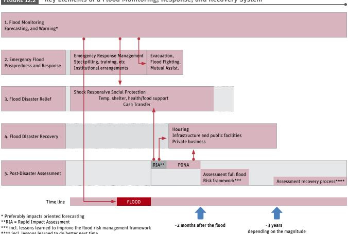
Key Elements of a Flood Monitoring, Response, and Recovery System FIGURE 12.2
