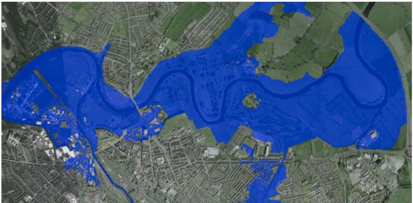
Figure 7 Example 100-year flood extent map for River Eden in Carlisle, UK. From http://web.sbe.hw.ac.uk/frmrc/index.htm (accessed 6 January 2014).
