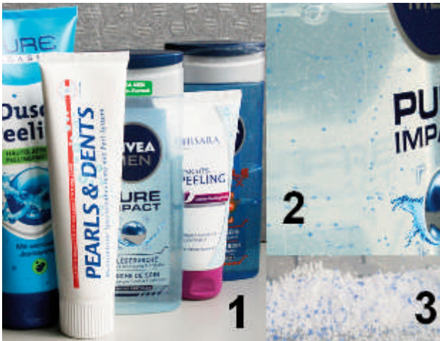
Photo 1: Personal care products containing microplastics (1), particles in shower gel (2), filtration residues of facial scrub (3).
