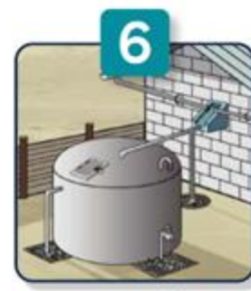
6 Rainwater collection and storage
