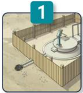
1 Dug well with a hand pump
