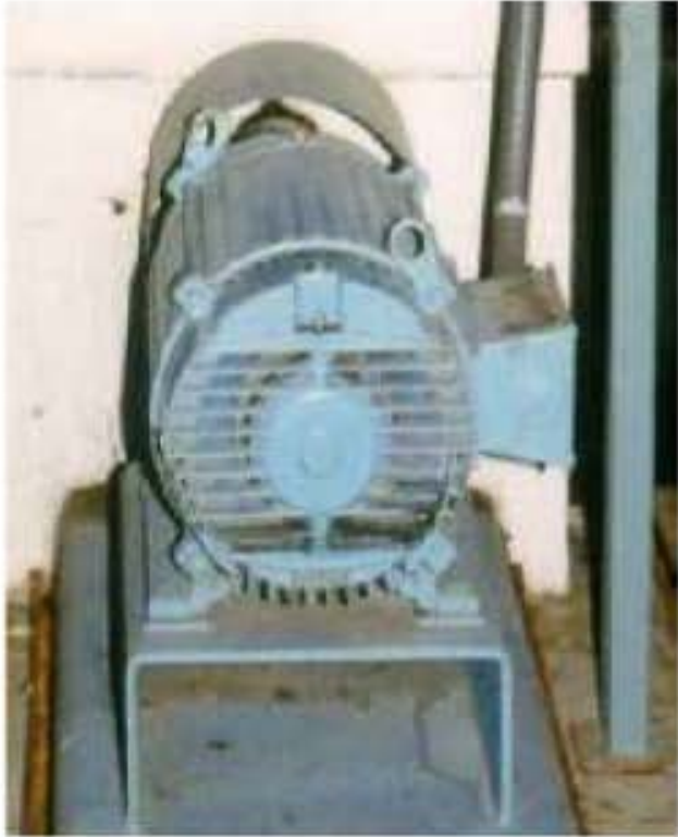
15 kW motor efficiency = 91%
